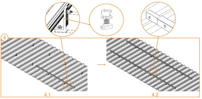
Connect the rail to the 13# hooks with the T-bolt M8\*28 and nut. Fasten to secure. Use the rail splice kit to connect the two rails with the two  $\phi 4.2*16$  self tapping bolts.
