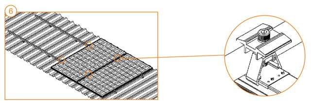
Put the second panel on the rail, fasten the mid clamps with inner hex bolts M8 at all locations where two panel meet .
