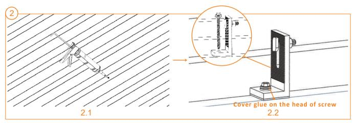
Backfill the pilot hole with sealant then fix the L-foot in place. Fix the L-foot in line. Then cover the glue on the head of screws to avoid rust.
