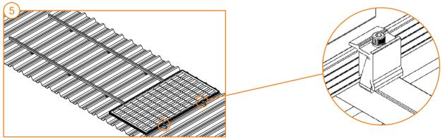
Put the first PV module on the two parallel rails ,fasten the end clamp with inner hex bolts M8 to secure one side of the panel .then slot two mid clamp on the rail.
