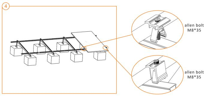
Install panels onto rails by fastening mid and end clamps.
