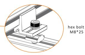
Connect rail to the beams by hex bolts M8\*25 (1 flat washer, 1 spring washer, and 1 nut);
