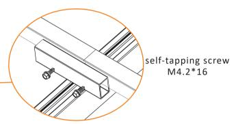
use rail splice kit to connect 2 rails by self-tapping screws M4.2\*16.
