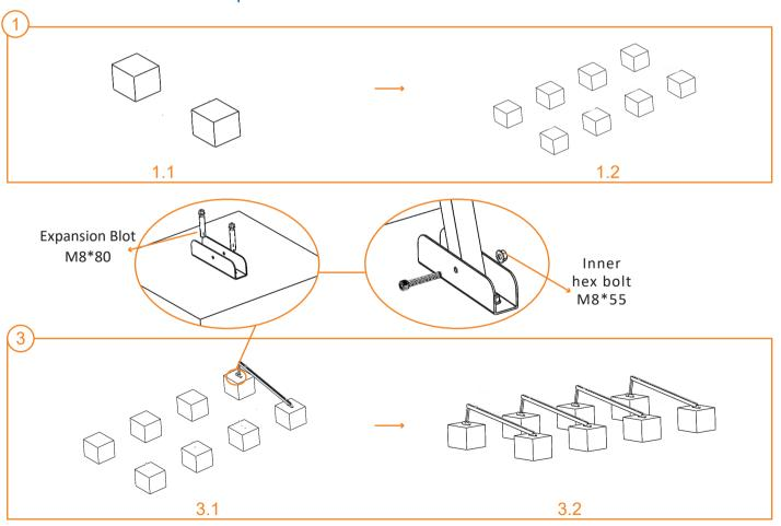
Connect the two bases to concrete block by Expansion Bolt set (1 flat washer, 1 spring washer, 1 nut); M8: tighten torque is 15N.m; safe torque is 20N.m;
