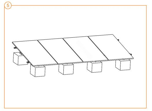
Double-check to make sure all bolts are fastened tight after installing all the panels.
